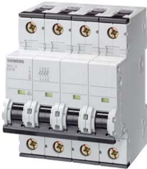
CIRCUIT BREAKER 400V 6KA, 4-POLE, C, 63A, D=70MM
